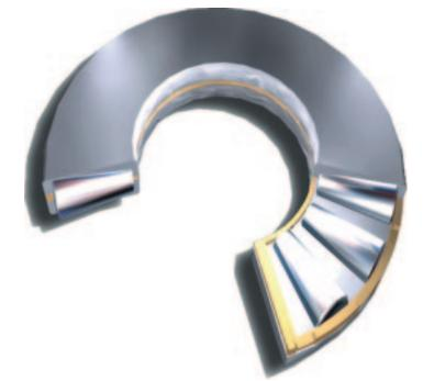
Rollway Tapered Roller Thrust Bearings are engineered for efficiency and longevity under the harshest industrial conditions. These rugged, dependable bearings feature true rolling motion, with the vertex of the conical sections meeting at the bearing axis.
