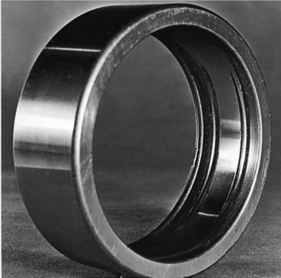
Figure 21 LUBRICATION FAILURE — RACEWAY
