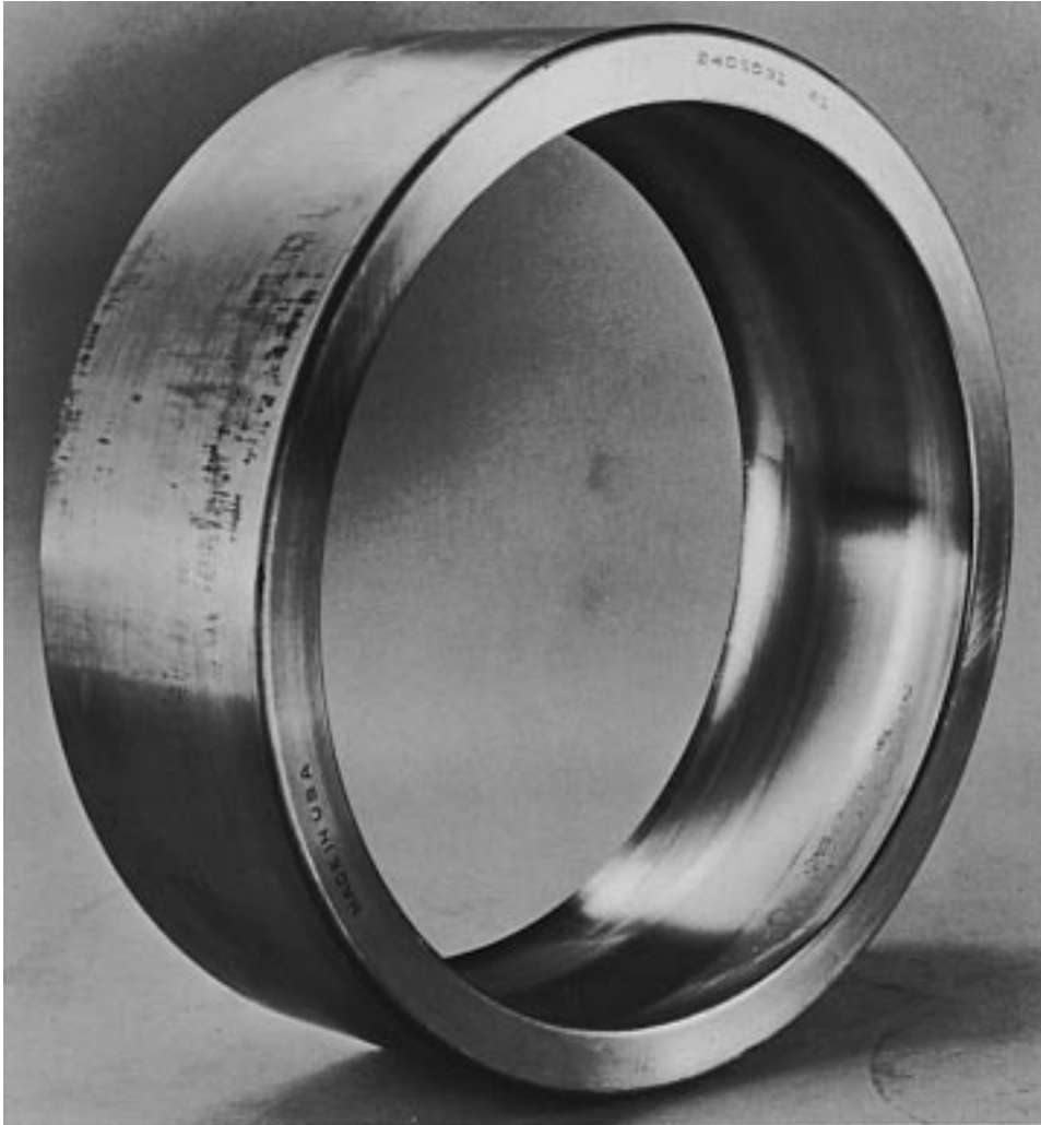
Figure 26 LUBRICATION FAILURE — OUTER RING
