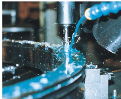
Special CNC machining centers drill bolt holes for mounting.
