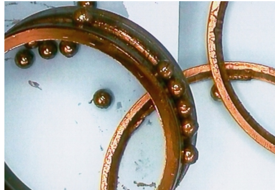
Water has penetrated into the bearing and has caused corrosion
